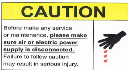
Figure 3. Disconnect Power label
