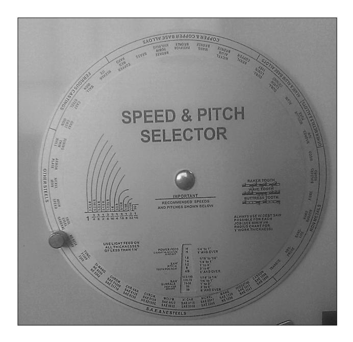
Select saw blades in relationship to the thickness of materials. The following suggestions are a rule of thumb to consider when selecting a blade.
