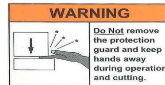
Figure 14. Guarding label – do not remove guarding & keep hands away from point of operation
