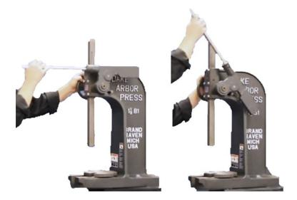
CAUTION: NEVER PULL THE PRESS HANDLE PAST THE HORIZONTAL POSITION! To avoid personal injury and damaging the press only pull until the handle is horizontal, then return the handle back up as far as it allows before bringing the handle back down. This ensures that the pawl fully engages with the gear teeth to prevent tooth damage and gear slippage that can cause harm to the machine and worker. Examples above show the ideal minimum and maximum handle positions.
