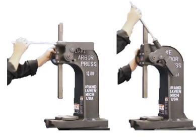
CAUTION: NEVER PULL THE PRESS HANDLE PAST THE HORIZONTAL POSITION! To avoid personal injury and damaging the press only pull until the handle is horizontal, then return the handle back up as far as it allows before bringing the handle back down. This ensures that the pawl fully engages with the gear teeth to prevent tooth damage and gear slippage that can cause harm to the machine and worker. Examples above show the ideal minimum and maximum handle positions.
